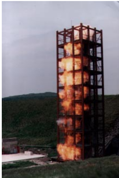
Figure 8: Explosion test in a bucket elevator, showing how the explosion propagates the length of the elevator in spite of the explosion vents (photo courtesy of the Health & Safety Laboratories).
