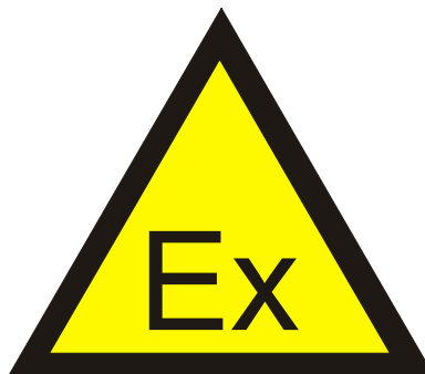
Figure 12: Sign prescribed by Directive 1999/92/EC to indicate hazardous areas in plant.
