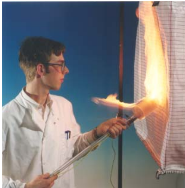
Photo 3: Gas Probe Incendivity Test
