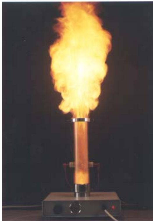
Photo 1: Minimum Ignition Energy test.
