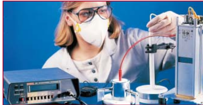
Resistivity and Charge Relaxation Time Testing
