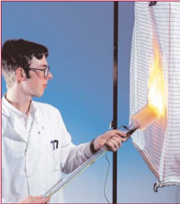
FIBC Testing: Gas probe showing ignition by static discharge
